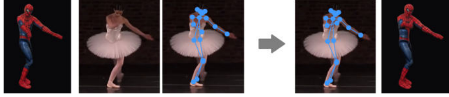
Figure 5.14. Editing an incorrectly detected pose to match the pose reference frame and regenerating the frame with the corrected pose
